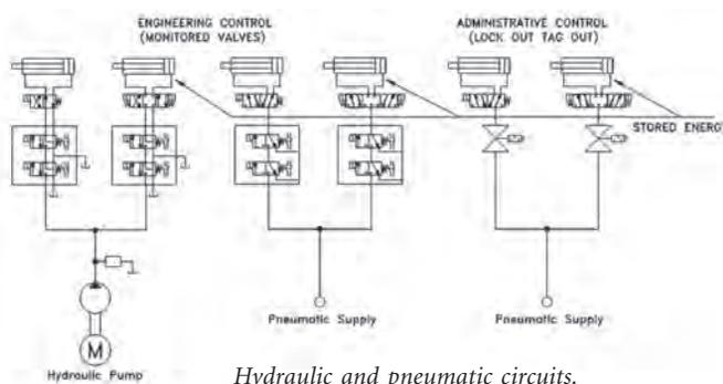
minor maintenance and breakdown scenarios, the stored energy is most dangerous in these inadvertent operating conditions due to the potential of the circuit being disassembled and the fittings being undone and stored energy being suddenly released to atmosphere.
